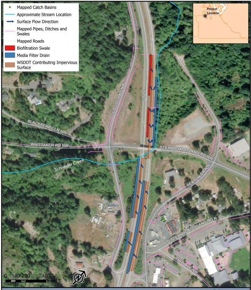
Schneider Creek Biofiltration Swales and Media Filter Drains
